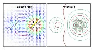
The panel on the left displays an electric field vector plot. The arrows in the field plot represent the direction and the colors represent the magnitude of the electric field.
